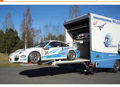
The DH-LSU.40 is a powerful lift for **heavy loads positioned at an unfavourable centre of gravity** (further away from the rear end of the vehicle).
