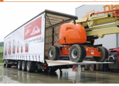
The heavy duty lift DH-LSU.90 is designed for **extreme lift capacities from 7,500 to 9,000 kg** and is mainly used for the transport of heavy machinery, forklifts, agricultural tractors etc...
