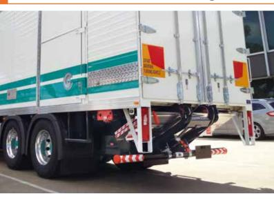
The DH-RC.15 is the ideal fold-away lift for **medium-duty** commercial vehicles. It is equipped with a wedged platform, offering a **level ride** from the vehicle floor to the ground (and vice versa), including automatic tilt at ground level.
