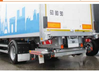
In comparison to the standard slider lifts DH-SM(R), the various DH-SO... lifts are equipped with a **double folded platform**: their platform is folded twice and rests on the lift arms when stowed away in travel position. Hence these DH-SO... lifts are specially designed for installation on **commercial vehicles with a too short overhang** to mount standard slider lifts with single folded platform (e.g. semi-trailers with rear steering axle, and centre-axle trailers).
